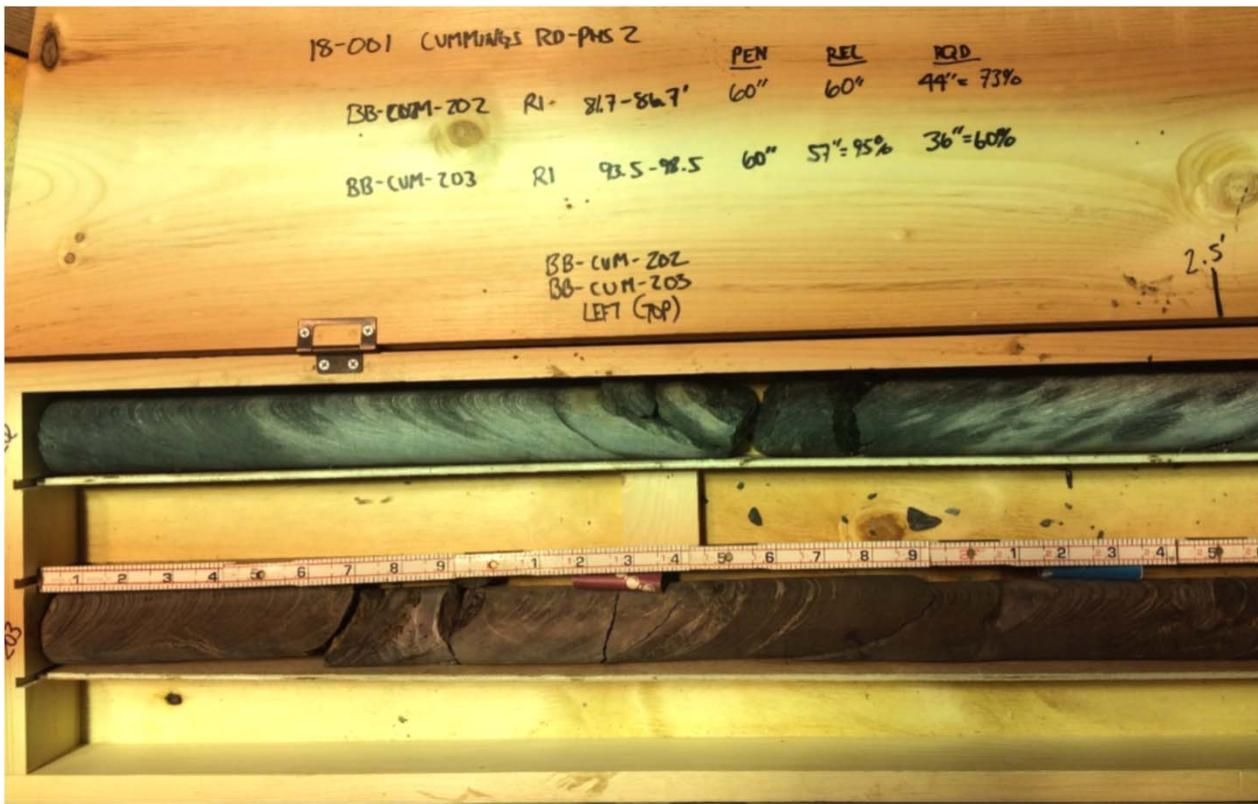
Photo 1: Core box containing rock core from test borings BB-CUM-202 & -203 left side of core box (top portion of cores).
