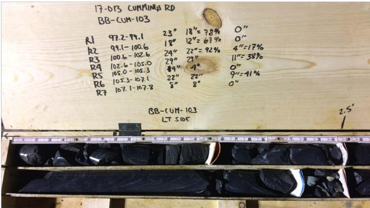
Photo 1: Core box containing wetted rock core from test boring BB-CUM-103 left side of core box (top portion of cores).
