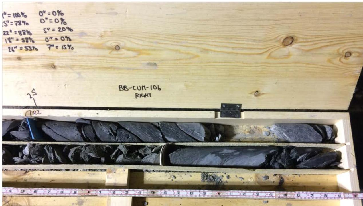
Photo 4: Core box containing dried rock core from test boring BB-CUM-106 – right side of core box (bottom portion of cores).
