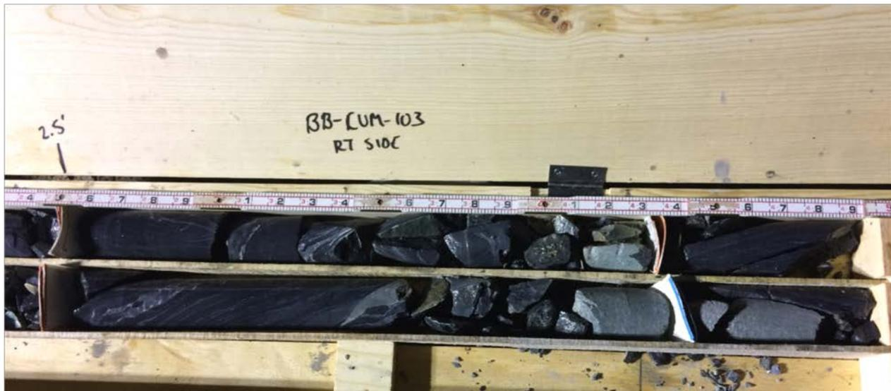
Photo 2: Core box containing wetted rock core from test boring BB-CUM-103 – right side of core box (bottom portion of cores).
