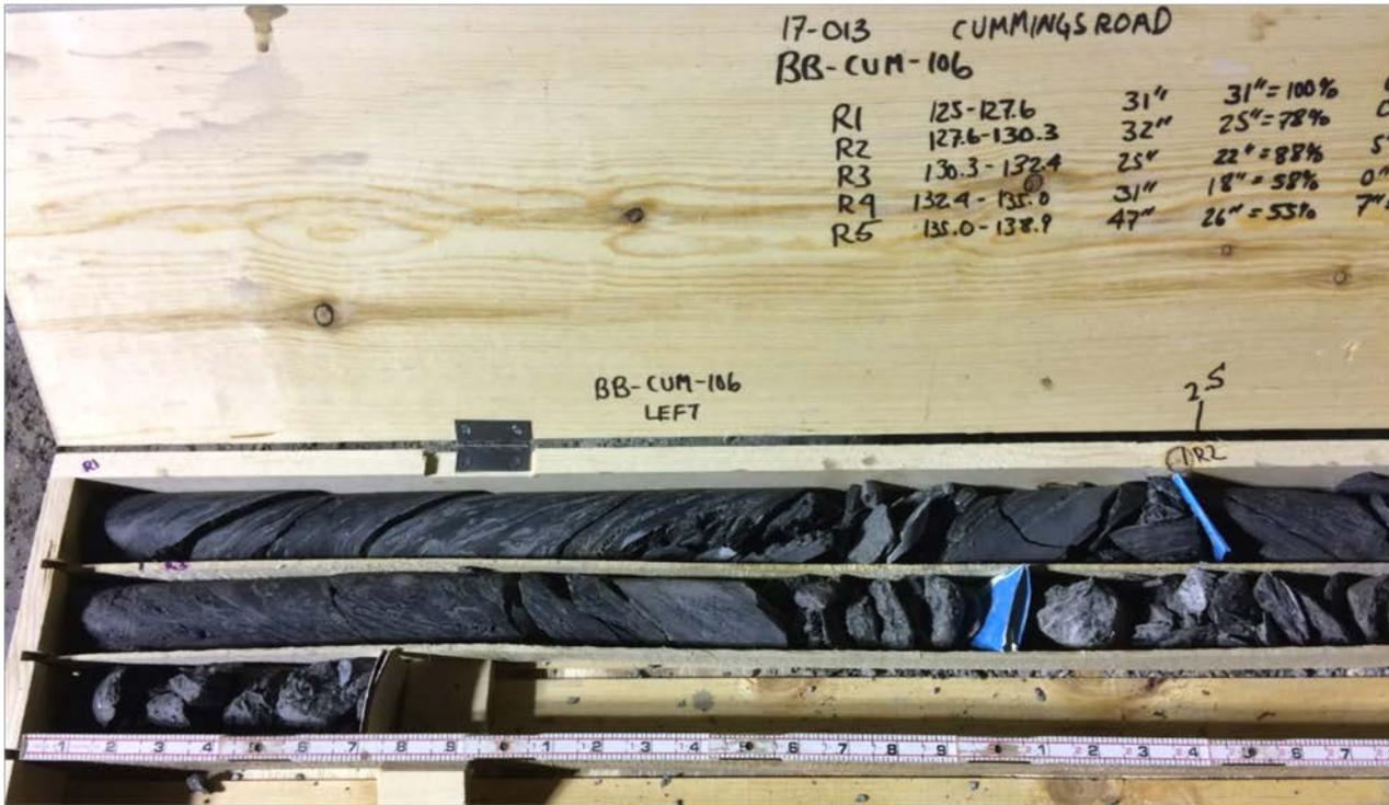
Photo 3: Core box containing dried rock core from test boring BB-CUM-106 left side of core box (top portion of cores).
