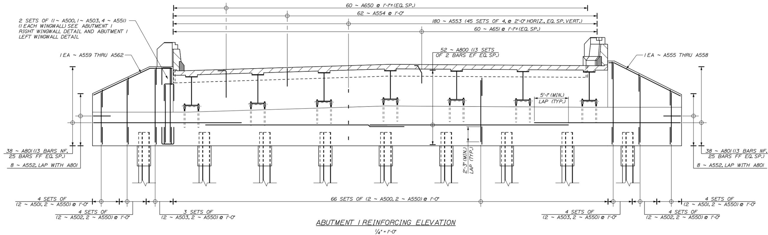
ABUTMENT 1 REINFORCING ELEVATION
