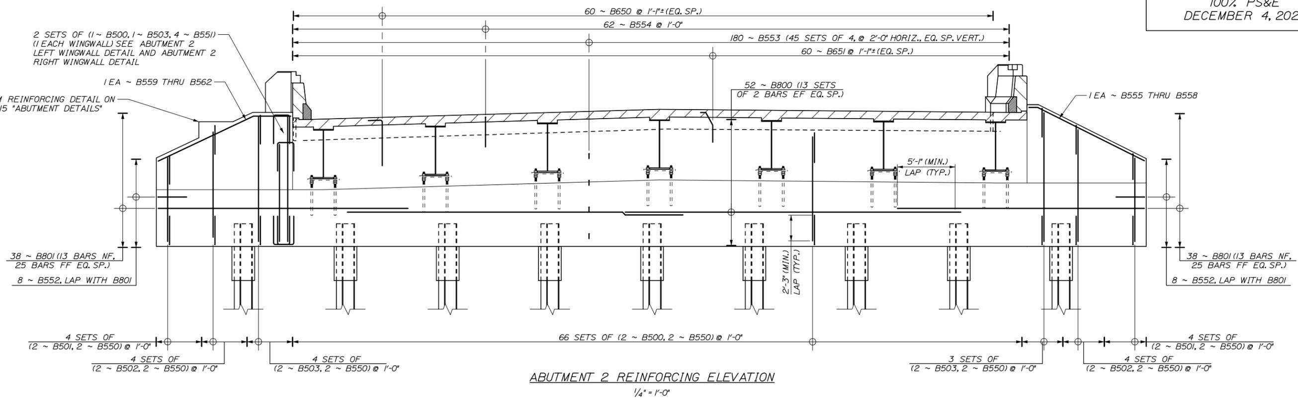
ABUTMENT 2 REINFORCING ELEVATION
