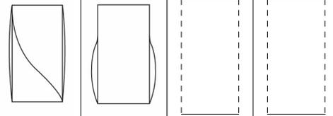
**THIELSCH: RESULTS OF UNCONFINED COMPRESSION LABORATORY TESTS
