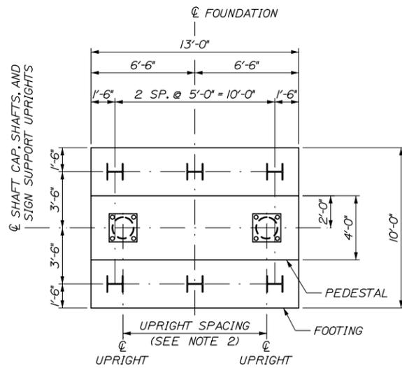
FOUNDATION - MASONRY PLAN
