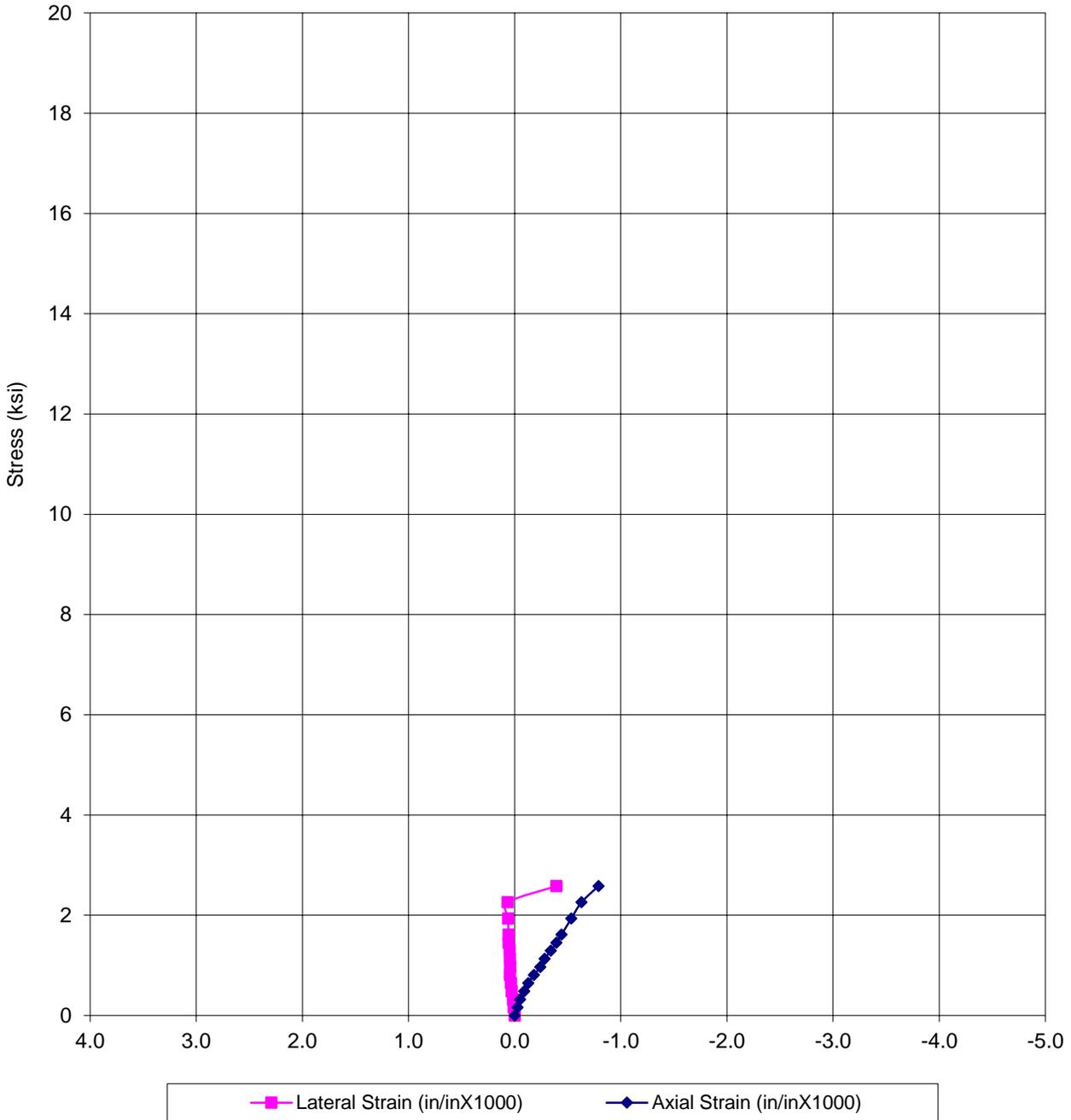
**Rock Unconfined Compression Testing - ASTM D7012**
