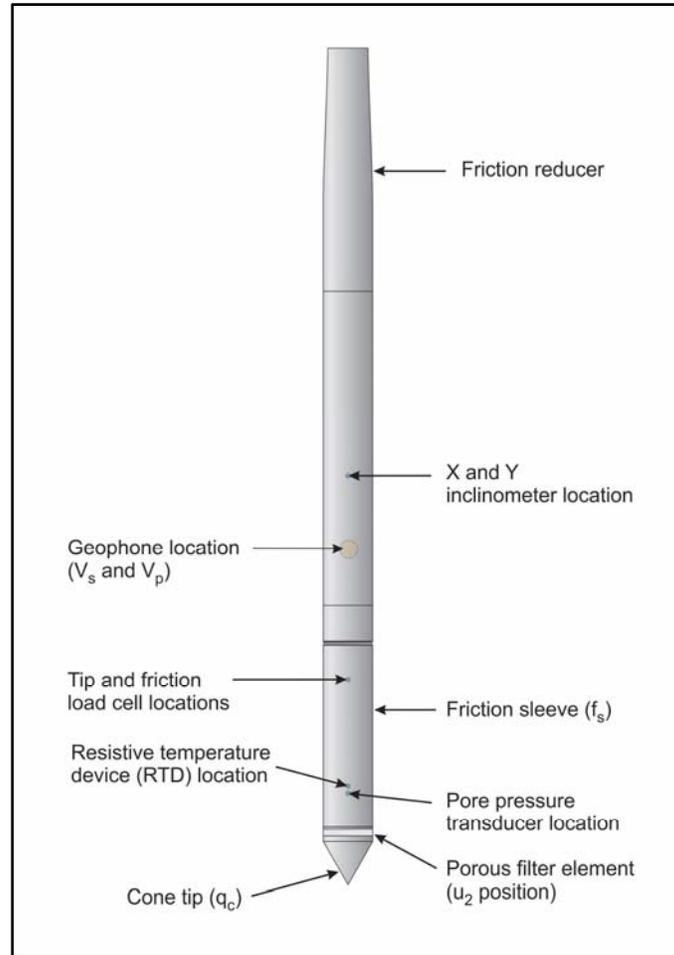
Figure CPTu. Piezocone Penetrometer (15 cm<sup>2</sup>)
