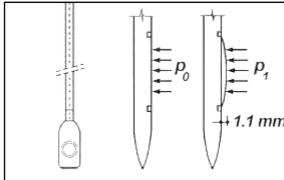
Figure DMT-2. Flat plate dilatometer  $p_0$  and  $p_1$
