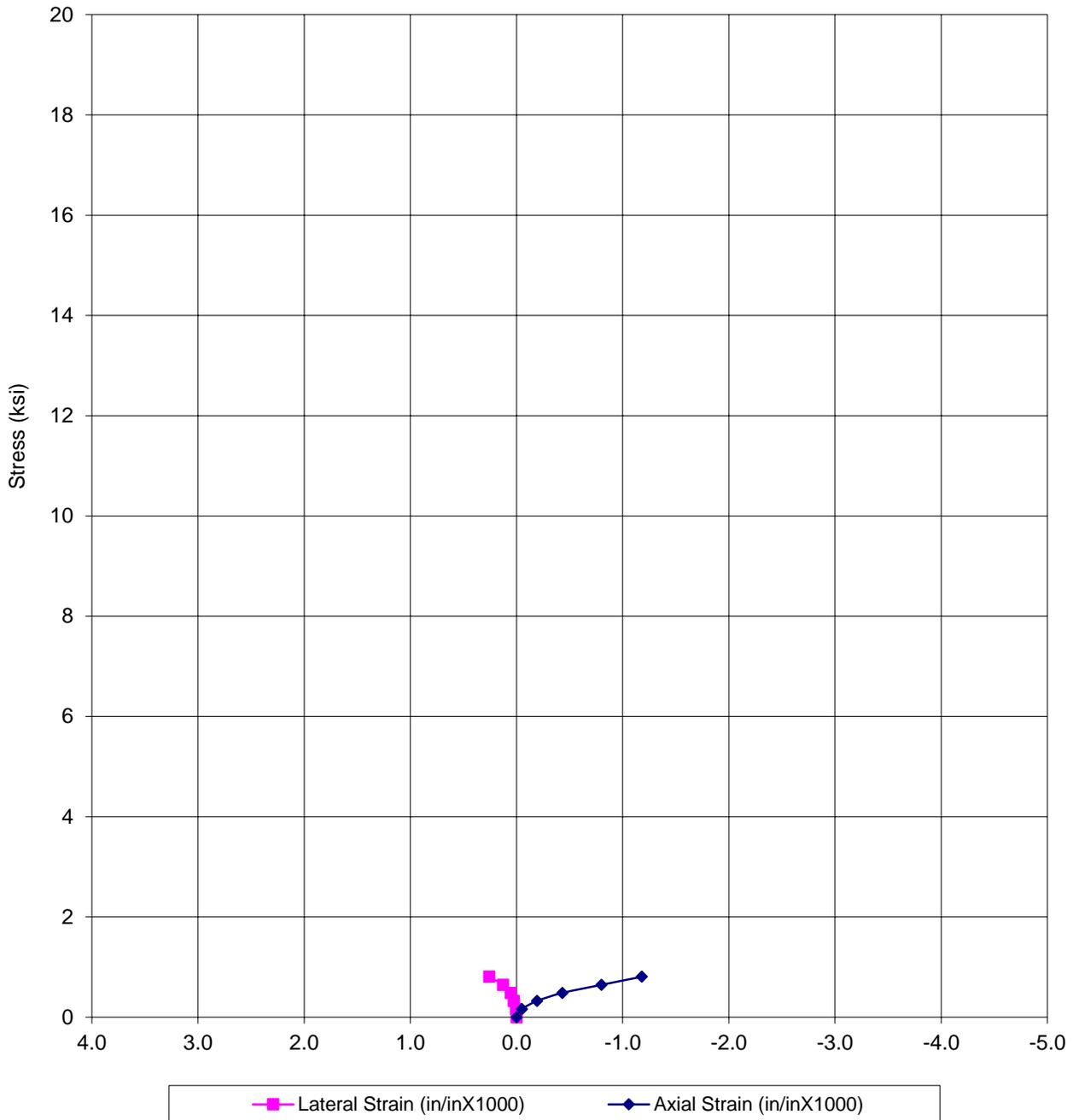
**Rock Unconfined Compression Testing - ASTM D7012**
