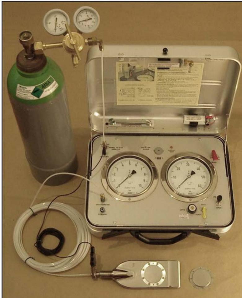
Figure DMT-1. Flat plate dilatometer system
