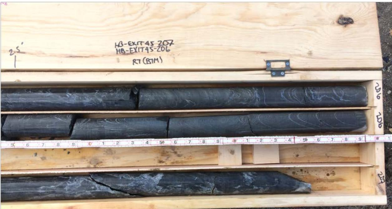
Photo 4: Core box containing wetted rock core from test borings HB-EXIT45-206 and -207 – right side of core box (bottom portion of cores).
