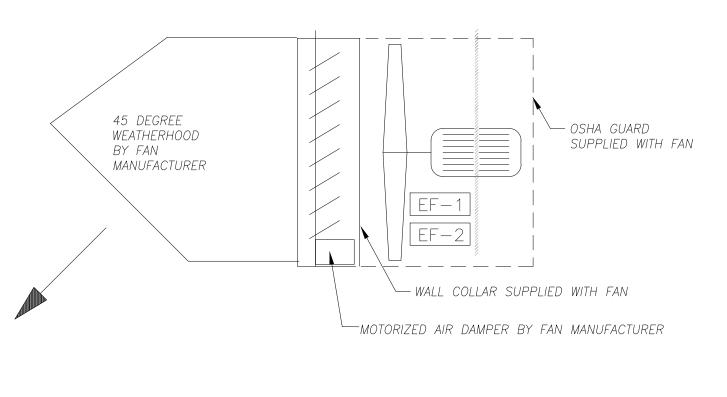
PITCH DUCTWORK UP FROM LOUVER FOR AT LEAST 6" – SEAL BOTTOM, SIDES AND CONNECTION TO LOUVER
