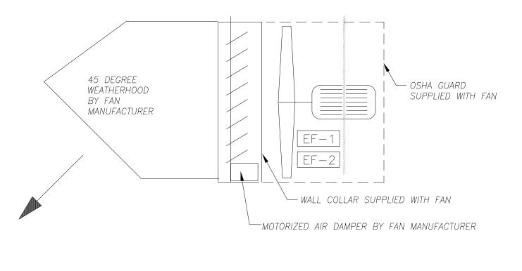
EXHAUST FAN DETAIL SECTION NO SCALE
