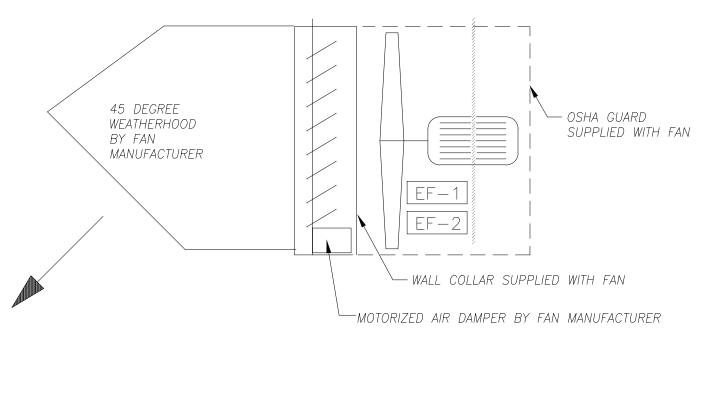
EXHAUST FAN DETAIL SECTION NO SCALE
