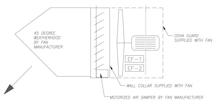
EXHAUST FAN DETAIL SECTION NO SCALE
