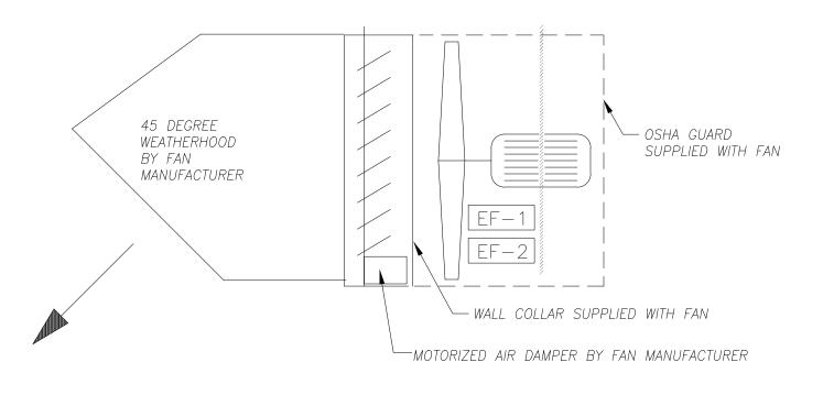
EXHAUST FAN DETAIL SECTION NO SCALE
