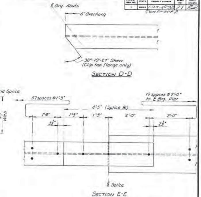
Note: Add 6" to beam lengths for overhang at abutments.
