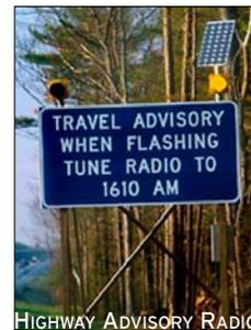
motorists to tune their radios to 1610 AM to receive real-time turnpike information. Prerecorded messages are continually broadcast to provide information about traffic conditions, weather, and construction zones. The communications center has the ability to control and quickly update messages. The
