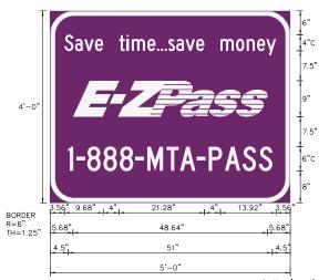
SIGN NUMBER SP-22 WIDTH x HGHT. 5'-0" x 4'-0" BORDER WIDTH 1.25" 6" CORNER RADIUS Ground MOUNTING BACKGROUND TYPE: Reflective COLOR: Purple LEGEND/BORDER TYPE: Reflective COLOR: White/White
