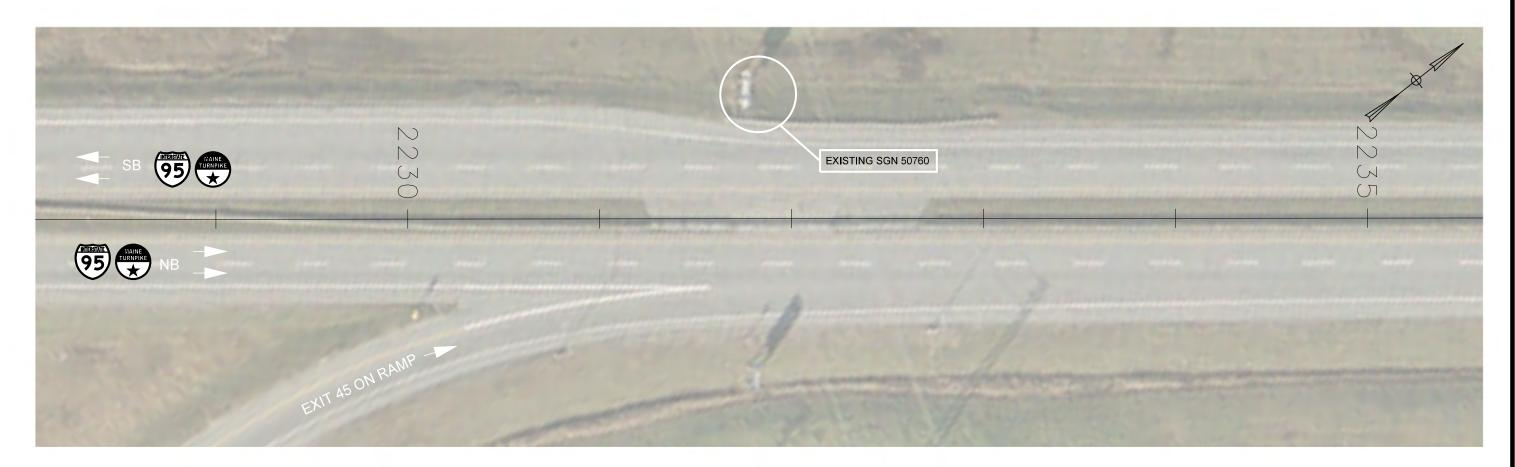
INSTALL NEW SHEET ALUMINUM OVERLAY OL-2 ON EXISTING SIGN
