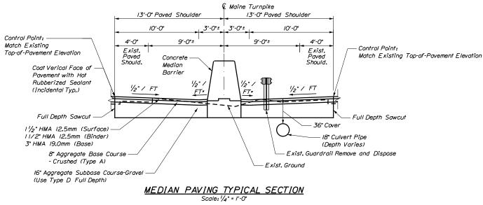
\* - Slopes At Concrete Median Barrier Face May Be Adjusted To Maintain Required Barrier Height
