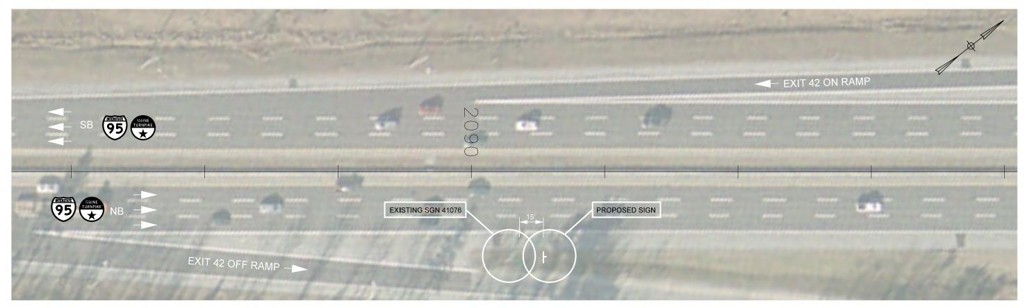
INSTALL NEW SIGN ON NEW SUPPORTS 15 FEET BEHIND EXISTING SIGN
