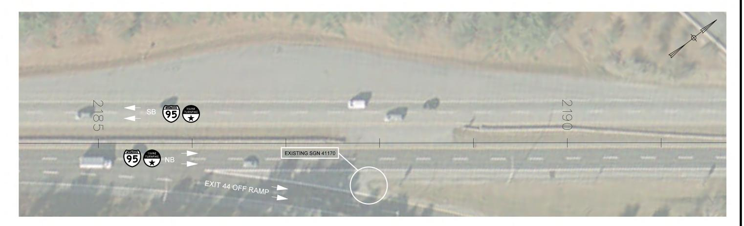
INSTALL NEW SIGN ON EXISTING SUPPORT TWO INCHES ABOVE THE HINGE PLATE
