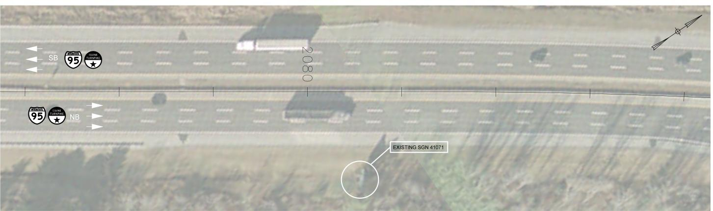
INSTALL NEW SIGN ON EXISTING SUPPORTS 2 INCHES ABOVE HINGE PLATE
