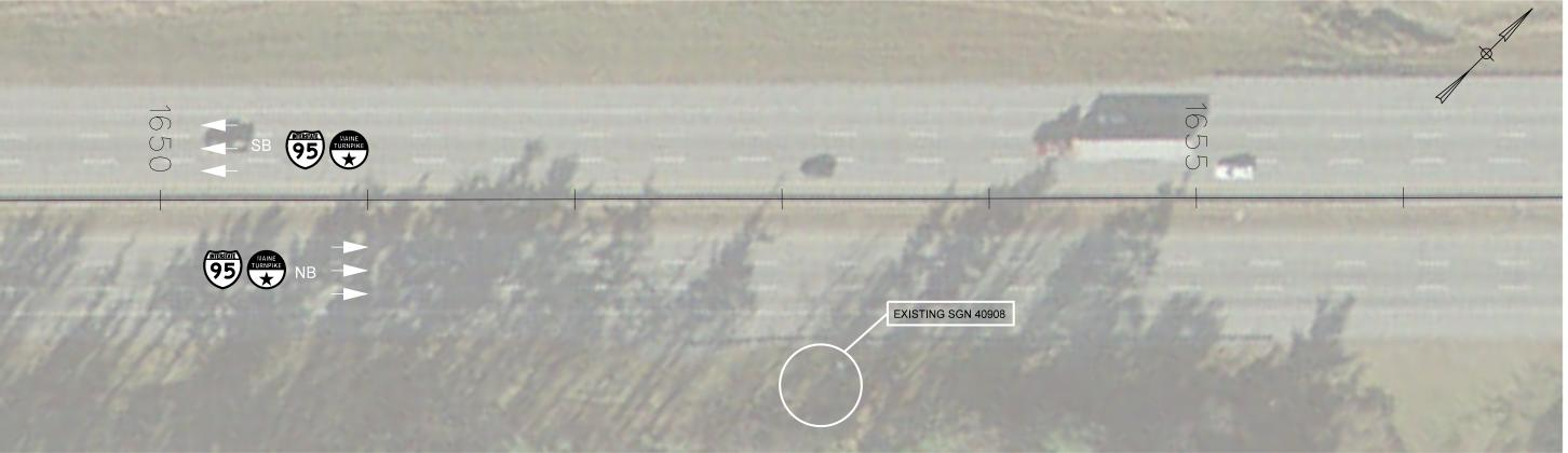
INSTALL NEW SIGN ON EXISTING SUPPORTS. MOUNT TOP OF SIGN WITH THE TOP OF THE SUPPORTS
