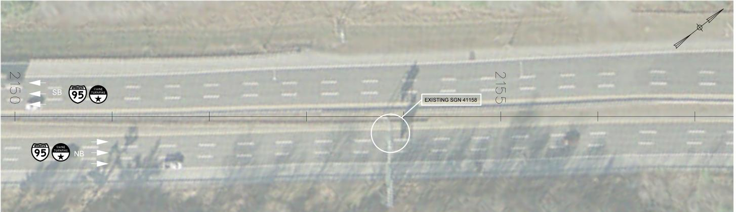
INSTALL NEW SIGN ON EXISTING OVERHEAD SIGN STRUCTURE WITH BOTTOM ALIGNED WITH ADJACENT SIGN
