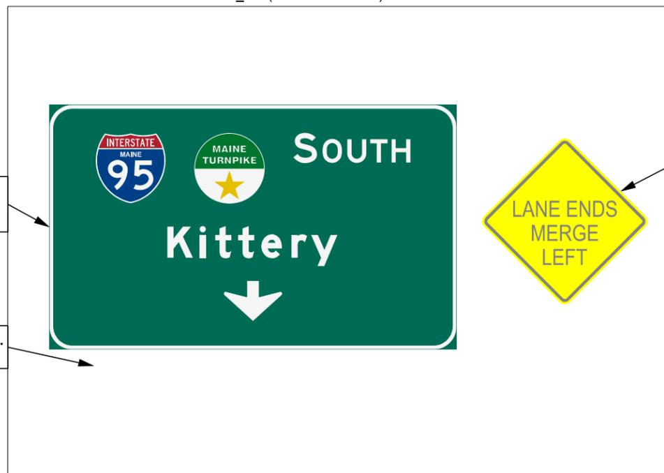
INSTALL NEW W9-2 SIGN TWO FEET AWAY FROM MTA SIGN 6363 ON EXISTING OVERHEAD SIGN STRUCTURE. VERTICALLY CENTER W9-2 TO THE ADJACENT SIGN
