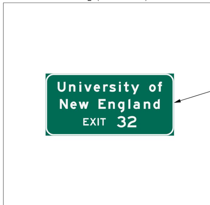
INSTALL NEW SIGN ON EXISTING SUPPORTS MOUNT TOP OF SIGN WITH TOP OF SUPPORTS
