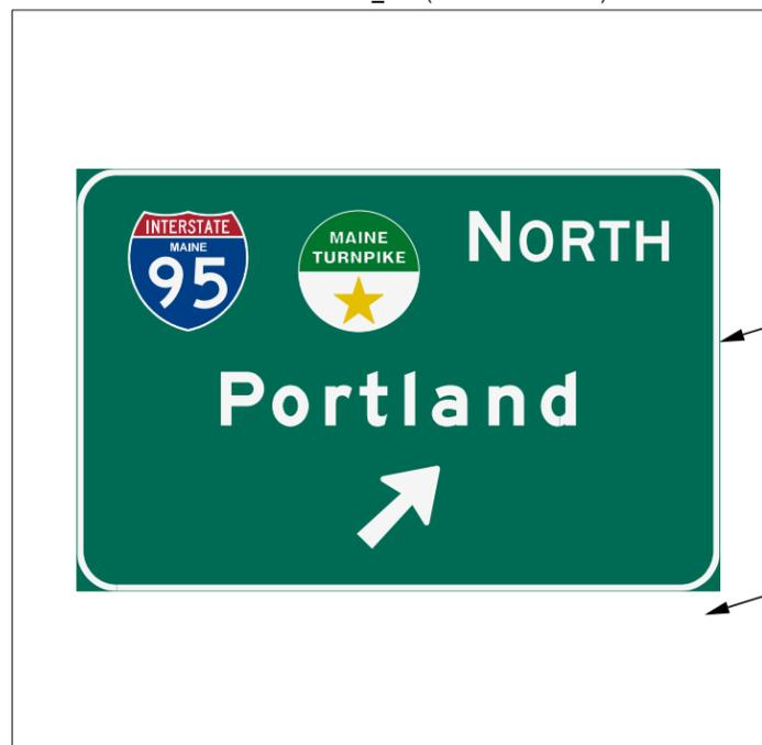
INSTALL NEW SIGN ON EXISTING OVERHEAD SIGN STRUCTURE WITH BOTTOM ALIGNED WITH ADJACENT SIGN
