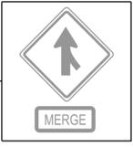
REINSTALL ORIGINAL W4-1 WITH SUPPLEMENTAL SIGN AT STA 2410+98
