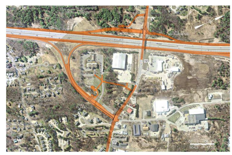
Figure 11.5 Route 112/Maine Turnpike Ramp Intersection Improvements Concept A6
