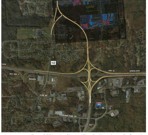
Figure 6.6 Diverging Diamond Signalized Interchange Configuration
