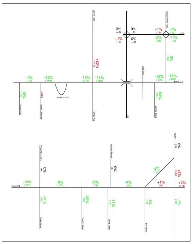
Figure 7.12 PM Peak Hour Comparison between A5 and 2040 No-Build Traffic Volume
