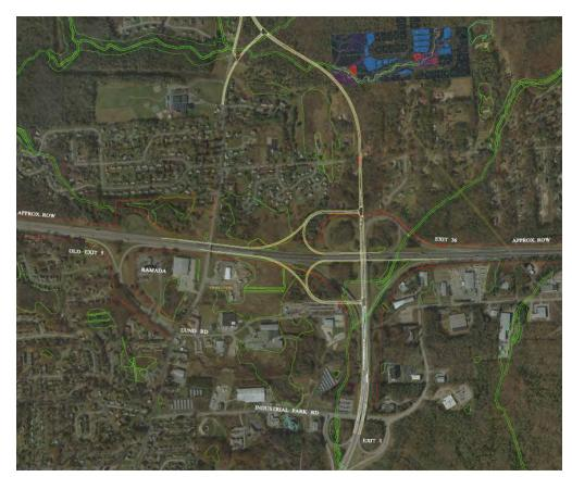
Figure 6.5 Partial Cloverleaf Signalized Interchange Configuration
